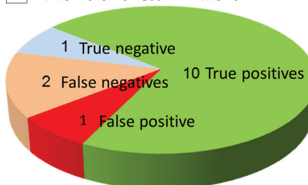
Figure 5. An example of statistical analysis of the RPI results from the Ceiba drilling campaign. (a) True positives, in which the seismic predicted sand and was correct, are in green; true negatives, in which the seismic correctly predicted no reservoir, are in blue; false positives, in which the seismic wrongly predicted reservoir, are in red; and false negatives, in which the seismic wrongly predicted the absence of reservoir, are in yellow. (b) The drilling campaign involved 14 wells, color coded according to the Boston square in (a). (c) Pie-chart representation of the results of (b). Figure modified, after Blangy et al. (2014).
